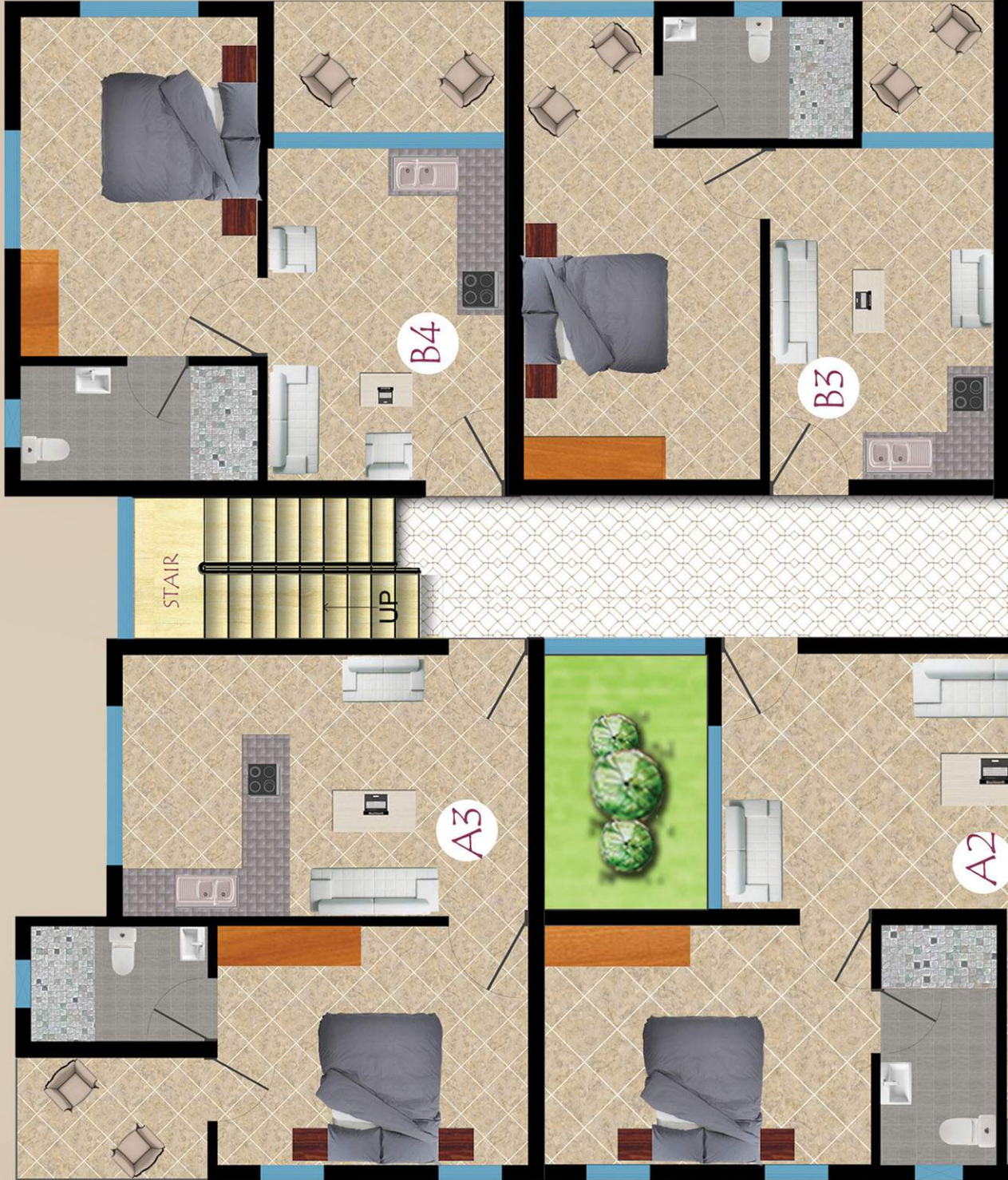
TYPICAL FLOOR LAYOUT - First and Second Floor
